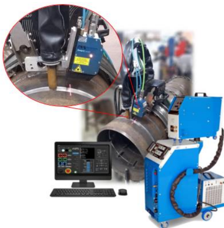
Figure 1 – Components of the orbital welding system developed in this study.
